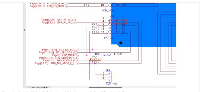
Figure 2. P0\_23(ADC0\_0, J13-3) used in this example in LPC55S16\_EVK
